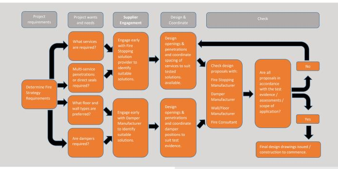
The building should be designed around the tested firestop solutions that are available.
